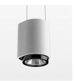
Suspended luminaire with LED, rated life of the LED L80/B10 > 50000 h, colour rendering index CRI > 96, chromaticity tolerance 3 SDCM (initial), LED hybrid technology, 3D silicone lens to reduce the proportion of scattered light, reflector with circular light distribution pattern, reflector pure aluminium 99,99% in MIRO-Silver®, segmented and faceted, exchangeable reflector unit in high-sheen black plastic, with glass cover, luminaire housing die-cast aluminium, powder-coated, stratowhite
