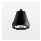
Suspended luminaire with LED, rated life of the LED L80/B10 > 50000 h, colour rendering index CRI > 96, chromaticity tolerance 2 SDCM (initial), rotation-symmetrical reflector with circular light distribution pattern, reflector pure aluminium 99,99% in MIRO-Silver®, segmented and faceted, 3D lens silicon to reduce the proportion of scattered light, luminaire head die-cast aluminium, powder-coated, stratoblack
