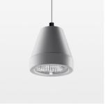
Suspended luminaire with LED, rated life of the LED L80/B10 > 50000 h, colour rendering index CRI > 90, chromaticity tolerance 3 SDCM (initial), rotation-symmetrical reflector with circular light distribution pattern, reflector pure aluminium 99,99% in MIRO-Silver®,segmented and faceted, 3D lens silicon to reduce the proportion of scattered light, luminaire head die-cast aluminium, powder-coated, stratosilver
