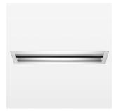
recessed luminaire with LED, rated life of the LED L80/B10 > 50000 h, color rendering index CRI > 90, chromaticity point tolerance 3 SDCM (initial), Reflector with asymerical light distribution pattern, 99.99% pure aluminium reflector made of MIRO-SILVER®, aluminium luminaire housing and frame, anodized, separate driver unit.
