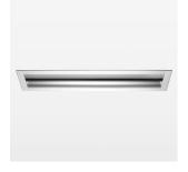
recessed luminaire with LED, rated life of the LED L80/B10 > 50000 h, color rendering index CRI > 80, chromaticity point tolerance 3 SDCM (initial), Reflector with asymerical light distribution pattern, 99.99% pure aluminium reflector made of MIRO-SILVER®, aluminium luminaire housing and frame, anodized, separate driver unit.
