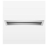
recessed luminaire with LED, rated life of the LED L80/B10 > 50000 h, color rendering index CRI > 80, chromaticity point tolerance 3 SDCM (initial), Reflector with asymerical light distribution pattern, 99.99% pure aluminium reflector made of MIRO-SILVER®, aluminium luminaire housing and frame, anodized, separate driver unit.
