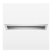
Recessed lumionaire for grid ceiling with LED, rated life of the LED L80/B10 > 50000 h, color rendering index CRI > 80, chromaticity point tolerance 3 SDCM (initial), Reflector with asymerical light distribution pattern, 99.99% pure aluminium reflector made of MIRO-SILVER®, aluminium luminaire housing and frame, anodized, separate driver unit.
