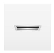
Recessed luminaire with LED, rated life of the LED L80/B10 > 50000 h, colour rendering index CRI > 90, chromaticity tolerance 3 SDCM (initial), reflector with asymmetrical light distribution pattern, reflector pure aluminium 99,99% in MIRO-Silver®, luminaire housing aluminium, aluminium, separate driver
