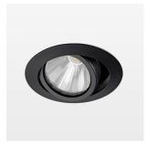
Recessed luminaire with LED, rated life of the LED L80/B10 > 50000 h, colour rendering index CRI > 96, chromaticity tolerance 2 SDCM (initial), rotation-symmetrical reflector with circular light distribution pattern, reflector pure aluminium 99,99% in MIRO-Silver®, segmented and faceted, 3D lens silicon to reduce the proportion of scattered light, die-cast aluminium, powder-coated, rotation angle , swivel angle +25° / -25°, stratoblack,
