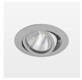
Recessed luminaire with LED, rated life of the LED L80/B10 > 50000 h, colour rendering index CRI > 90, chromaticity tolerance 3 SDCM (initial), rotation-symmetrical reflector with circular light distribution pattern, reflector pure aluminium 99,99% in MIRO-Silver®, segmented and faceted, 3D lens silicon to reduce the proportion of scattered light, die-cast aluminium, powder-coated, rotation angle, swivel angle +25° / -25°, stratosilver,
