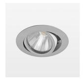
Recessed luminaire with LED, rated life of the LED L80/B10 > 50000 h, colour rendering index CRI > 80, chromaticity tolerance 3 SDCM (initial), rotation-symmetrical reflector with circular light distribution pattern, reflector pure aluminium 99,99% in MIRO-Silver®, segmented and faceted, 3D lens silicon to reduce the proportion of scattered light, die-cast aluminium, powder-coated, rotation angle, swivel angle +25°/-25°, stratosilver,
