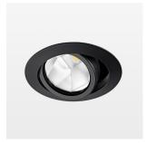
Recessed luminaire with LED, rated life of the LED L80/B10 > 50000 h, colour rendering index CRI > 96, chromaticity tolerance 2 SDCM (initial), reflector with oval light distribution pattern, reflector pure aluminium 99,99% in MIRO-Silver®, segmented, die-cast aluminium, powder-coated, rotation angle , swivel angle  $+25^{\circ}$  /  $-25^{\circ}$ , stratoblack,
