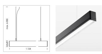
Light band with LED, rated life of the LED L80/B50 > 50000 h, colour rendering index CRI > 80, reflector with homogeneous light distribution pattern, lens optics made of PMMA, luminaire insert sheet steel, powder-coated, black
