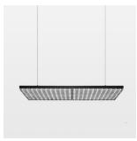
Suspended luminaire with LED, rated life of the LED L80/B50 > 50000 h, colour rendering index CRI > 80, chromaticity tolerance 3 SDCM (initial), double asymmetrical light distribution pattern, lens made of PMMA, luminaire housing sheet steel, powder-coated, matt black, power supply via suspension cables.
