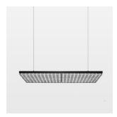
Suspended luminaire with LED, rated life of the LED L80/B50 > 50000 h, colour rendering index CRI > 80, chromaticity tolerance 3 SDCM (initial), double asymmetrical light distribution pattern, lens made of PMMA, luminaire housing sheet steel, powder-coated, matt black, power supply via suspension
