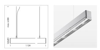
Light band with LED, rated life of the LED L80/B50 > 50000 h, colour rendering index CRI > 80, reflector with homogeneous light distribution pattern, lens optics made of PMMA, luminaire insert sheet steel, powder-coated, silver
