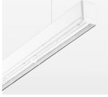
Light band with LED, rated life of the LED L80/B50 > 50000 h, colour rendering index CRI > 80, reflector with homogeneous light distribution pattern, lens optics made of PMMA, luminaire insert sheet steel, powder-coated, white
