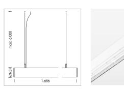
Light band with LED, rated life of the LED L80/B50 > 50000 h, colour rendering index CRI > 80, reflector with homogeneous light distribution pattern, lens optics made of PMMA, luminaire insert sheet steel, powder-coated, white
