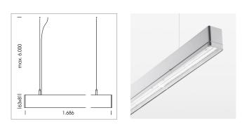
Light band with LED, rated life of the LED L80/B50 > 50000 h, colour rendering index CRI > 80, reflector with homogeneous light distribution pattern, lens optics made of PMMA, luminaire insert sheet steel, powder-coated, silver
