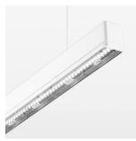
Light band with LED, rated life of the LED L80/B50 > 50000 h, colour rendering index CRI > 80, reflector with double asymmetrical light distribution pattern, lens optics made of PMMA, luminaire insert sheet steel, powder-coated, white
