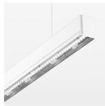
Light band with LED, rated life of the LED L80/B50 > 50000 h, colour rendering index CRI > 80, reflector with double asymmetrical light distribution pattern, lens optics made of PMMA, luminaire insert sheet steel, powder-coated, white
