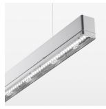
Light band with LED, rated life of the LED L80/B50 > 50000 h, colour rendering index CRI > 80, reflector with double asymmetrical light distribution pattern, lens optics made of PMMA, luminaire insert sheet steel, powder-coated silver
