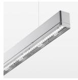
Light band with LED, rated life of the LED L80/B50 > 50000 h, colour rendering index CRI > 80, reflector with double asymmetrical light distribution pattern, lens optics made of PMMA, luminaire insert sheet steel, powder-coated, silver
