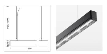
Light band with LED, rated life of the LED L80/B50 > 50000 h, colour rendering index CRI > 80, reflector with double asymmetrical light distribution pattern, lens optics made of PMMA, luminaire insert sheet steel, powder-coated, black
