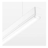
Light band with LED, rated life of the LED L80/B50 > 50000 h, colour rendering index CRI > 80, reflector with homogeneous light distribution pattern, lens optics made of PMMA, luminaire insert sheet steel, powder-coated, white
