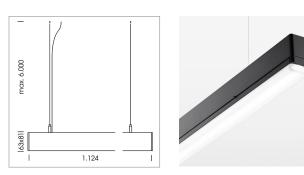
Light band with LED, rated life of the LED L80/B50 > 50000 h, colour rendering index CRI > 80, reflector with homogeneous light distribution pattern, lens optics made of PMMA, luminaire insert sheet steel, powder-coated, black
