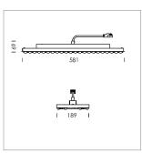
Lay in luminaire with LED, rated life of the LED L80/B50 > 50000 h, colour rendering index CRI > 80, chromaticity tolerance 3 SDCM (initial), double asymmetrical light distribution pattern, lens made of PMMA, luminaire housing sheet steel, powder-coated, matt white
