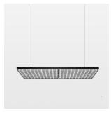
Suspended luminaire with LED, rated life of the LED L80/B50 > 50000 h, colour rendering index CRI > 80, chromaticity tolerance 3 SDCM (initial), double asymmetrical light distribution pattern, lens made of PMMA, luminaire housing sheet steel, powder-coated, matt black, power supply via suspension cobles.
