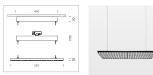
Suspended luminaire with LED, rated life of the LED L80/B50 > 50000 h, colour rendering index CRI > 80, chromaticity tolerance 3 SDCM (initial), double asymmetrical light distribution pattern, lens made of PMMA, luminaire housing sheet steel, powder-coated, matt black, power supply via suspension cables
