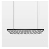
Suspended luminaire with LED, rated life of the LED L80/B50 > 50000 h, colour rendering index CRI > 80, chromaticity tolerance 3 SDCM (initial), double asymmetrical light distribution pattern, lens made of PMMA, luminaire housing sheet steel, powder-coated, matt black, power supply via suspension cables.
