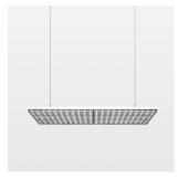
Suspended luminaire with LED, rated life of the LED L80/B50 > 50000 h, colour rendering index CRI > 80, chromaticity tolerance 3 SDCM (initial), double asymmetrical light distribution pattern, lens made of PMMA, luminaire housing sheet steel, powder-coated, matt white, power supply via suspension cables
