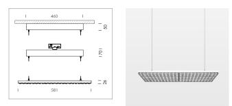
Suspended luminaire with LED, rated life of the LED L80/B50 > 50000 h, colour rendering index CRI > 80, chromaticity tolerance 3 SDCM (initial), double asymmetrical light distribution pattern, lens made of PMMA, luminaire housing sheet steel, powder-coated, matt white, power supply via suspension cables
