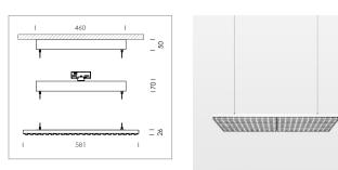
Suspended luminaire with LED, rated life of the LED L80/B50 > 50000 h, colour rendering index CRI > 80, chromaticity tolerance 3 SDCM (initial), double asymmetrical light distribution pattern, lens made of PMMA, luminaire housing sheet steel, powder-coated, matt white, power supply via suspension cables
