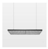
Suspended luminaire with LED, rated life of the LED L80/B50 > 50000 h, colour rendering index CRI > 80, chromaticity tolerance 3 SDCM (initial), wide, homogeneous light distribution pattern, TIR-lens made of PMMA, luminaire housing sheet steel, powder-coated, matt black, power supply via suspension cables
