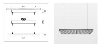
Suspended luminaire with LED, rated life of the LED L80/B50 > 50000 h, colour rendering index CRI > 80, chromaticity tolerance 3 SDCM (initial), wide, homogeneous light distribution pattern, TIR-lens made of PMMA, luminaire housing sheet steel, powder-coated, matt black, power supply via suspension cables
