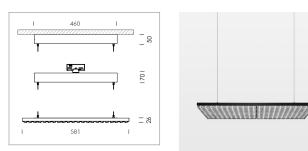
Suspended luminaire with LED, rated life of the LED L80/B50 > 50000 h, colour rendering index CRI > 80, chromaticity tolerance 3 SDCM (initial), extra wide, homogeneous light distribution pattern, TIR-lens made of PMMA, luminaire housing sheet steel, powder-coated, matt black, power supply via suspension cables
