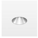
Recessed downlight, flush with ceiling with LED, rated life of the LED L80/B10 > 50000 h, colour rendering index CRI > 90, chromaticity tolerance 2 SDCM (initial), reflector with homogeneous light distribution pattern, diffuser lens, translucent, darklight reflector, aluminium, metallised, highgloss, luminaire head die-cast aluminium, black anodized black anodized, Ceiling plaster die-cast aluminum, trim plastic injection molding, black, separate driver unit
