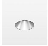
Recessed downlight, flush with ceiling with LED, rated life of the LED L80/B10 > 50000 h, colour rendering index CRI > 96, chromaticity tolerance 2 SDCM (initial), reflector with homogeneous light distribution pattern, diffuser lens, translucent, darklight reflector, aluminium, metallised, highgloss, luminaire head die-cast aluminium, black anodized black anodized, Ceiling plaster die-cast aluminum, trim plastic injection molding, black, separate driver unit
