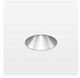
Recessed downlight, flush with ceiling with LED, rated life of the LED L80/B10 > 50000 h, colour rendering index CRI > 96, chromaticity tolerance 3 SDCM (initial), reflector with homogeneous light distribution pattern, diffuser lens, translucent, darklight reflector, aluminium, metallised, highgloss, luminaire head die-cast aluminium, black anodized black anodized, Ceiling plaster die-cast aluminum, trim plastic injection molding, black, separate driver unit
