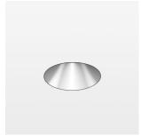
Recessed downlight, flush with ceiling with LED, rated life of the LED L80/B10 > 50000 h, chromaticity tolerance 3 SDCM (initial), reflector with homogeneous light distribution pattern, diffuser lens, translucent, darklight reflector, aluminium, metallised, highgloss, luminaire head die-cast aluminium, black angelized.
