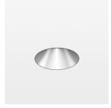
Recessed downlight, flush with ceiling with LED, rated life of the LED L80/B10 > 50000 h, colour rendering index CRI > 90, chromaticity tolerance 2 SDCM (initial), reflector with homogeneous light distribution pattern, diffuser lens, translucent, darklight reflector, aluminium, metallised, highgloss, luminaire head die-cast aluminium, black anodized black anodized, Ceiling plaster die-cast aluminum, trim plastic injection molding, black, separate driver unit
