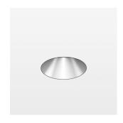
Recessed downlight, flush with ceiling with LED, rated life of the LED L80/B10 > 50000 h, chromaticity tolerance 2 SDCM (initial), reflector with homogeneous light distribution pattern, diffuser lens, translucent, darklight reflector, aluminium, metallised, highgloss, luminaire head die-cast aluminium, black anodized
