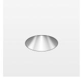
Recessed downlight, flush with ceiling with LED, rated life of the LED L80/B10 > 50000 h, chromaticity tolerance 3 SDCM (initial), reflector with homogeneous light distribution pattern, diffuser lens, translucent, darklight reflector, aluminium, metallised, highgloss, luminaire head die-cast aluminium, black anodized
