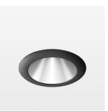
Recessed downlight with LED, rated life of the LED L80/B10 > 50000 h, colour rendering index CRI > 80, chromaticity tolerance 2 SDCM (initial), reflector with homogeneous light distribution pattern, diffuser lens, translucent, darklight reflector, aluminium, metallised, highgloss, luminaire head die-cast aluminium, powder-coated, mounting ring die-cast aluminum, front ring and coverblind plastic, black, separate driver unit
