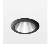
Recessed downlight with LED, rated life of the LED L80/B10 > 50000 h, colour rendering index CRI > 80, chromaticity tolerance 2 SDCM (initial), reflector with homogeneous light distribution pattern, diffuser lens, translucent, darklight reflector, aluminium, metallised, highgloss, luminaire head die-cast aluminium, powder-coated, mounting ring die-cast aluminum, front ring and coverblind plastic, black, separate driver unit
