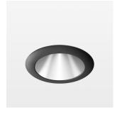
Recessed downlight with LED, rated life of the LED L80/B10 > 50000 h, colour rendering index CRI > 80, chromaticity tolerance 2 SDCM (initial), reflector with homogeneous light distribution pattern, diffuser lens, translucent, darklight reflector, aluminium, metallised, highgloss, luminaire head die-cast aluminium, powder-coated, mounting ring die-cast aluminum, front ring and coverblind plastic, black, separate driver unit
