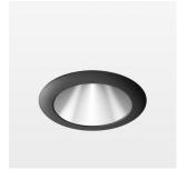
Recessed downlight with LED, rated life of the LED L80/B10 > 50000 h, colour rendering index CRI > 96, chromaticity tolerance 3 SDCM (initial), reflector with homogeneous light distribution pattern, diffuser lens, translucent, darklight reflector, aluminium, metallised, highgloss, luminaire head die-cast aluminium, powder-coated, mounting ring die-cast aluminum, front ring and coverblind plastic, black, separate driver unit
