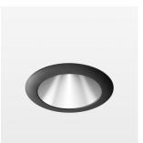
Recessed downlight with LED, rated life of the LED L80/B10 > 50000 h, chromaticity tolerance 2 SDCM (initial), reflector with homogeneous light distribution pattern, diffuser lens, translucent, darklight reflector, aluminium, metallised, highgloss, luminaire head die-cast aluminium, powder-coated, mounting ring die-cast aluminum, front ring and coverblind plastic, black, separate driver unit
