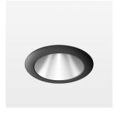
Recessed downlight with LED, rated life of the LED L80/B10 > 50000 h, chromaticity tolerance 3 SDCM (initial), reflector with homogeneous light distribution pattern, diffuser lens, translucent, darklight reflector, aluminium, metallised, highgloss, luminaire head die-cast aluminium, powder-coated, mounting ring die-cast aluminum, front ring and coverblind plastic, black, separate driver unit
