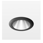
Recessed downlight with LED, rated life of the LED L80/B10 > 50000 h, colour rendering index CRI > 90, chromaticity tolerance 2 SDCM (initial), reflector with homogeneous light distribution pattern, diffuser lens, translucent, darklight reflector, aluminium, metallised, highgloss, luminaire head die-cast aluminium, powder-coated, mounting ring die-cast aluminum, front ring and coverblind plastic, black, separate driver unit
